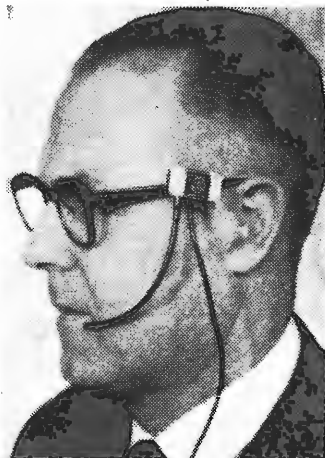
"Micro-miniature" headset from S. G. Brown Ltd. As can be seen a microphone boom is not needed with this headset, which weighs less than 1 oz.
