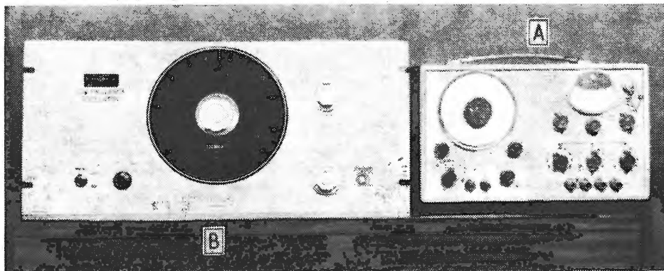
Fig. 15. Commercial Audio "Standard-signal" Generators: (A) Marconi TF2000 (transistorized); (B) W. G. Pye 11025.
